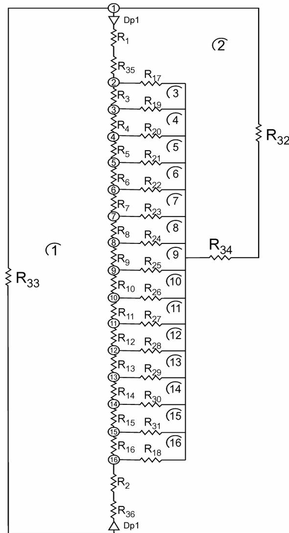
Figure 6. Resistance element network for hydrogenerator ventilation analysis.
