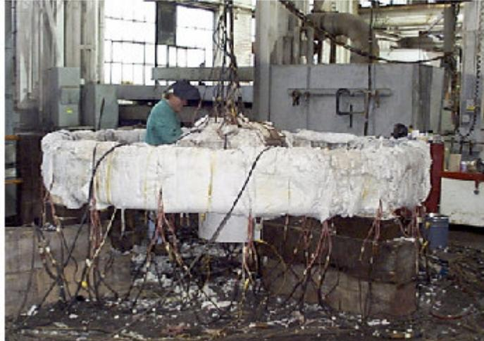
*Figure 4. Setup of spider for pre-heat and post-weld heat treatment.*
