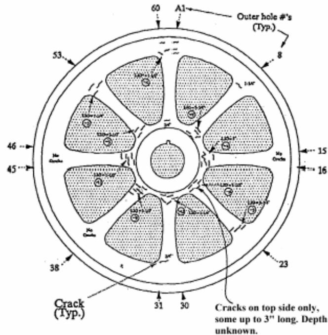
Figure 1. Shown above is an overall sketch of the spider arm and crack locations. Over 50 cracks in various lengths and depths were present on this machine. After this sketch was made, cracks were confirmed on both sides of the spider.
