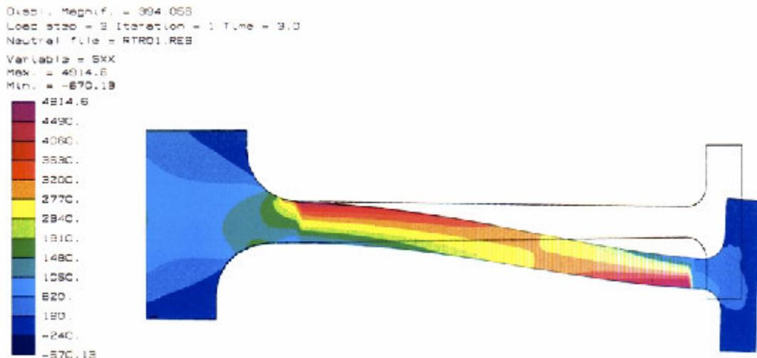
*Figure 3. Spider arm stress and deflection at overspeed.*
