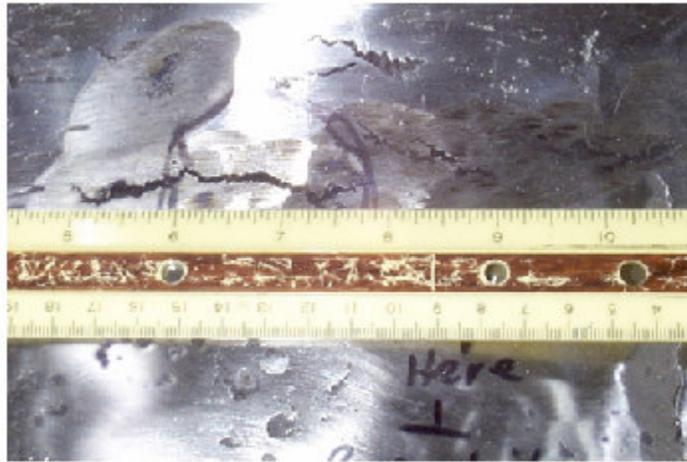
*Figure 2. Photograph of cracks in a typical spider arm. Most of the cracks were located at the transition area between the thick hub and the thinner spider arm.*
