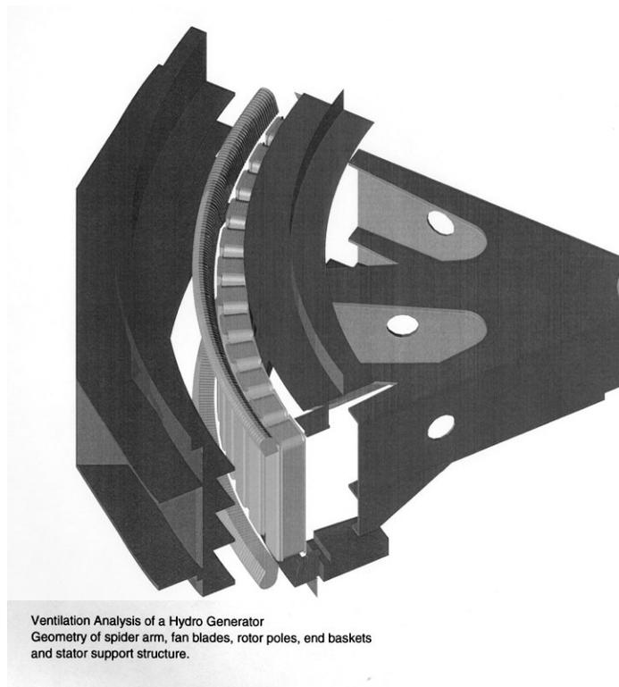
*Figure 7. CFD (Computational Fluid Dynamic) model of a hydrogenerator to analyze ventilation. Shown in this particular model is the spider arm, fan blades, rotor poles, stator end winding coils and the stator support structure.*
