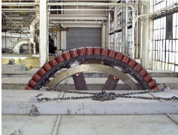
*Figure 5. Photograph of spider in National Electric Coil's balance pit. Pole pieces, as shown, are assembled on the spider.*
