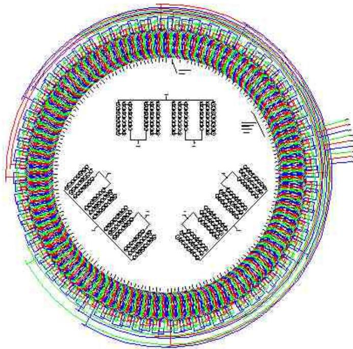
*Figure 9. Computer generated winding diagram for a hydrogenerator.*
