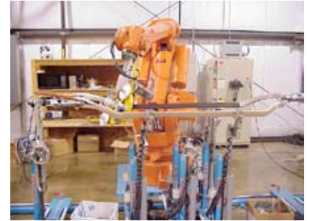
Automated application of groundwall tapes.
