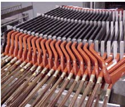
Precision-cut dummy core used for dimensional checks (all systems) and final factory cure for Systems I and II.
