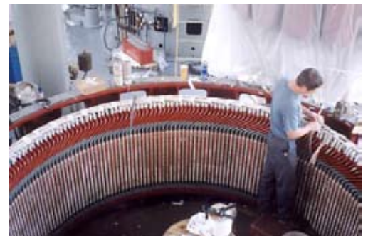
Top two photos show rewinds in progress using coils made with the NECCOPress™ Insulation system.
