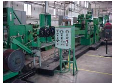
In production order: Above Copper wire drawn and rolled to specified size. Left: Application of strand insulation to conductor. Bottom Left: Robotic application of turn tape and subsequent looping of turns. Bottom Right: Forming of coil geometries.
