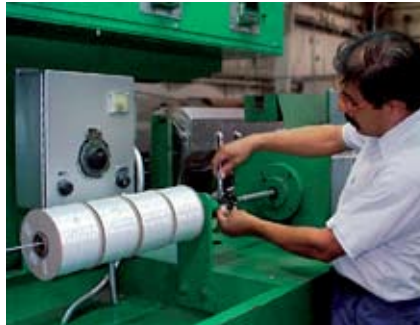
Top two photos show rewinds in progress using coils made with the NECCOPress™ Insulation system.
