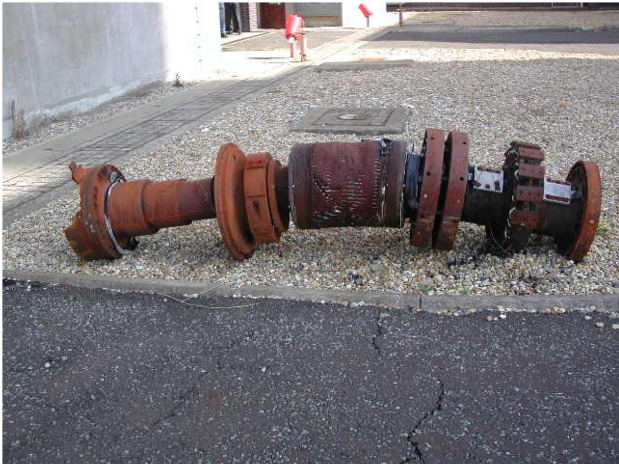
Figure 2: Damage to the exciter from the fire was extensive..
